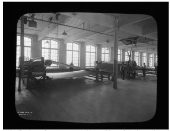
The final napping process used a machine with a large drum of green plant thistles secured to the drum which would lightly brush the surface of the felt. Each felt was inspected and repaired if necessary prior to shipping.
