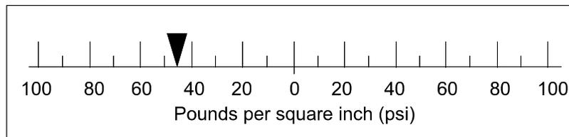
Which one of the following is most nearly the reading shown on the pressure gauge above?
