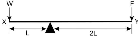
In the balance, or scale, system shown above, how much force (F) must be applied at point Y to balance the weight (W) at point X?
