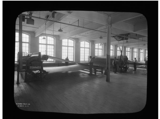
The final napping process used a machine with a large drum of green plant thistles secured to the drum which would lightly brush the surface of the felt. Each felt was inspected and repaired if necessary prior to shipping.
