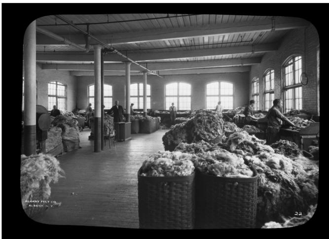
Raw wool was transferred to 'pickers' on the 3rd floor. Wool pickers separated different grades of wool from a single fleece. An apprenticeship of 3 years was required to qualify as an expert wool picker.
