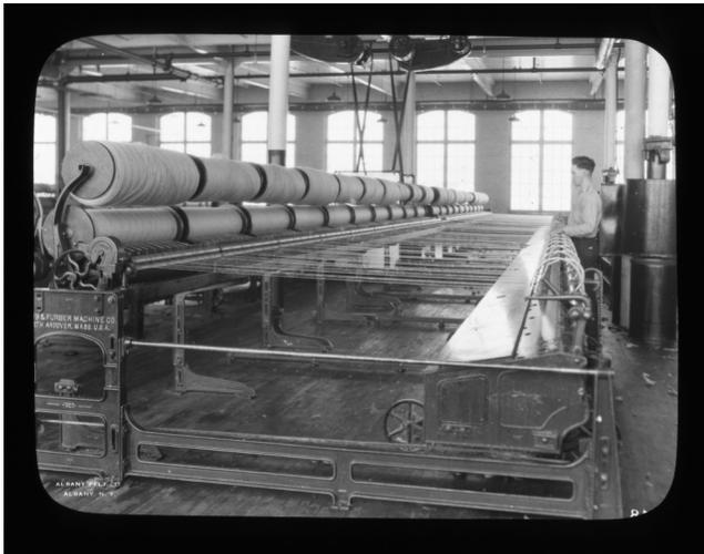
Large cylinders of 'carded' wool were sent to the Mule Spinning Machines which took up an entire wing of the building. Mule spinning gathered wool yarn and transferred it to smaller bobbins.
